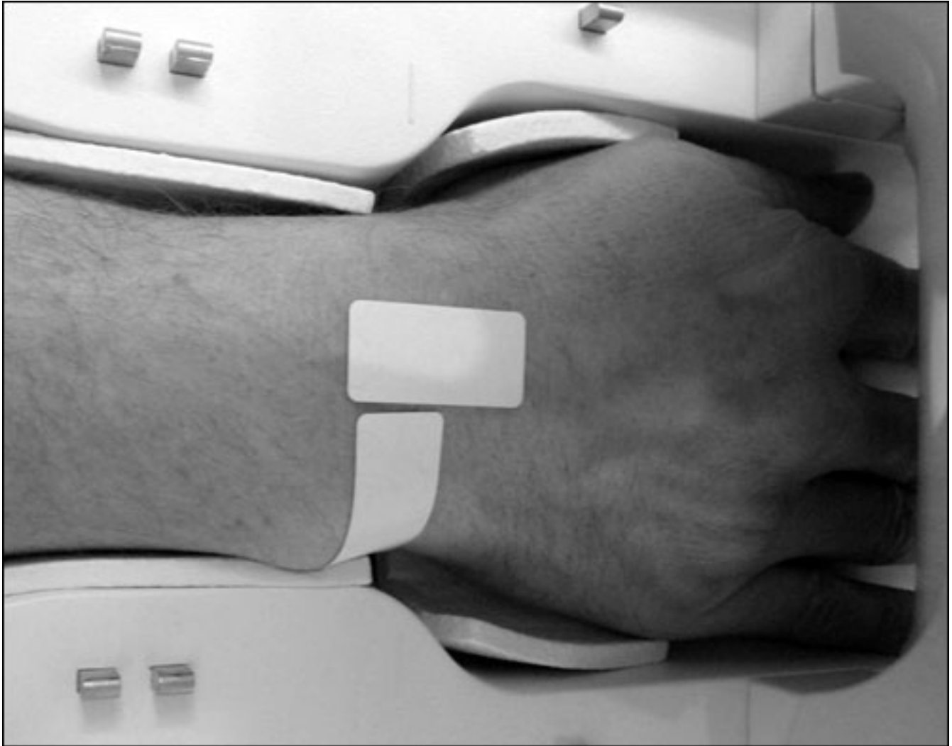
Two RFID tags were attached directly to the wrist of a volunteer and scanned by an MRI device.
